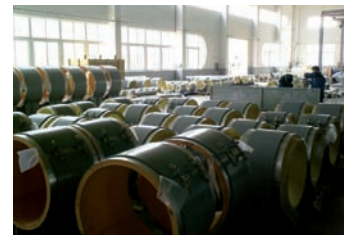
Preassembled cryogenic pipe supports
