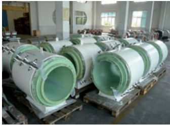
Preassembled cryogenic pipe supports
